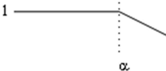
Figure 1-3: Single Pole Low Pass Filter Transfer Function H(s)
